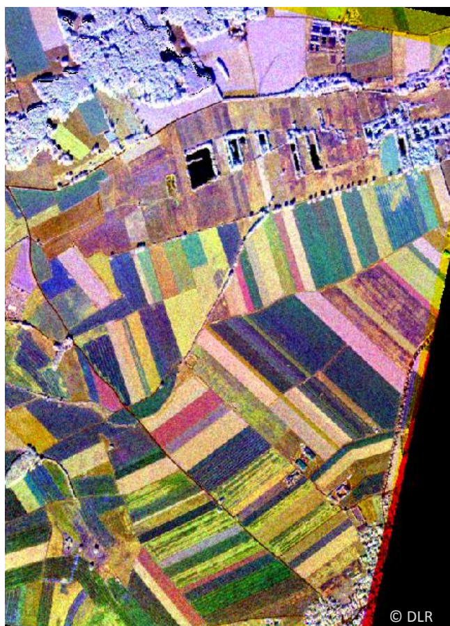
Fig.: X-VV / C-VV / L-VV composite (left) and crop type map (right)
