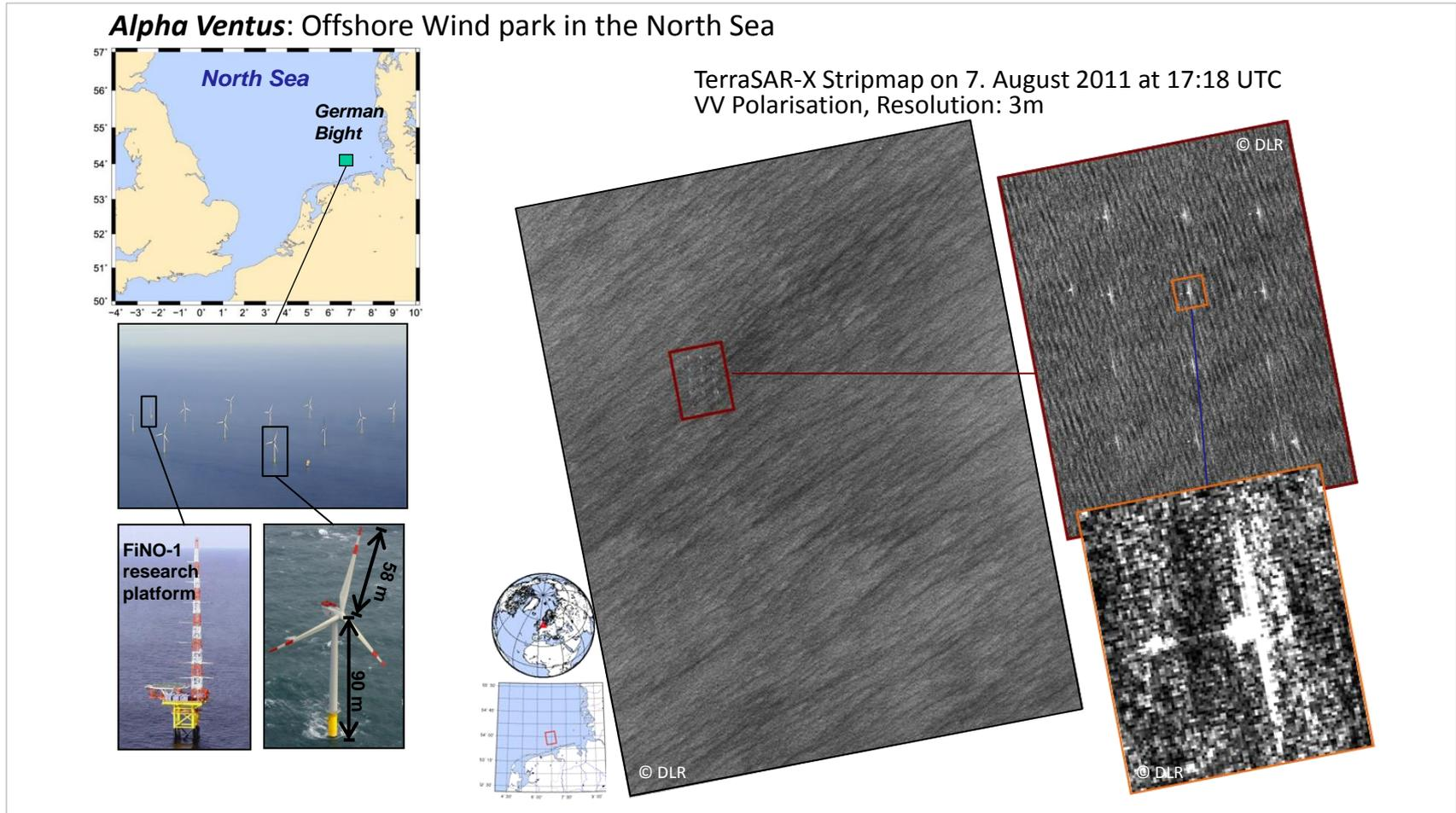
Fig. 17: Wind estimation from TerraSAR-X Stripmap image for *Alpha Ventus* Offshore Wind Park in the North Sea (© DLR, Li)
