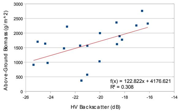
Figure A 5: The scatterplot and regression model derived from the ALOS PALSAR HV data adjusted for tide and the biomass field data. The regression model was used to estimate potential error due to tide level in the previous biomass calculation.
