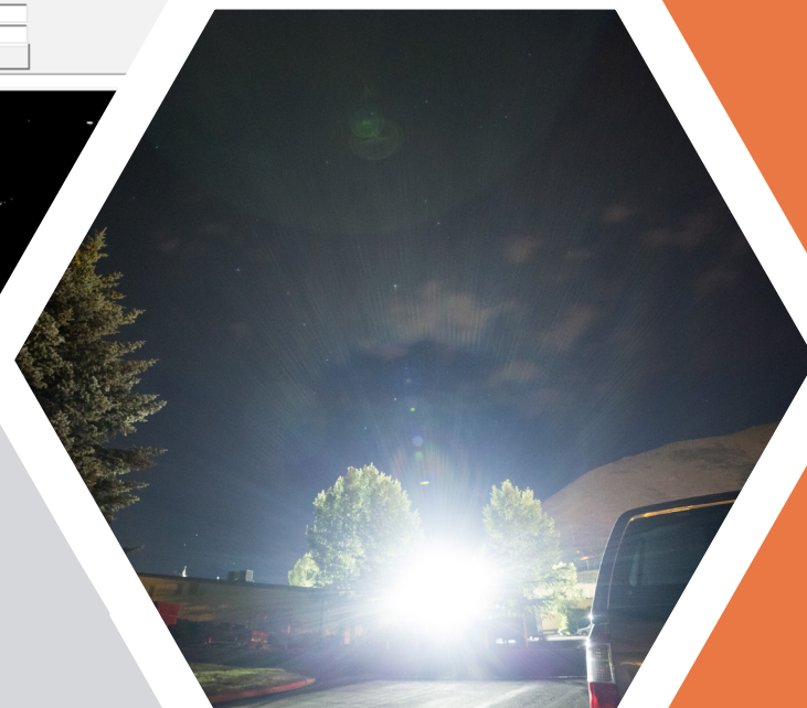
Fig. 4. Use minimum amount of lighting needed to illuminate target. In this case, excess light escapes into the sky, degrading nighttime visibility. > © Mike Cavaroc/Free Roaming Photography
