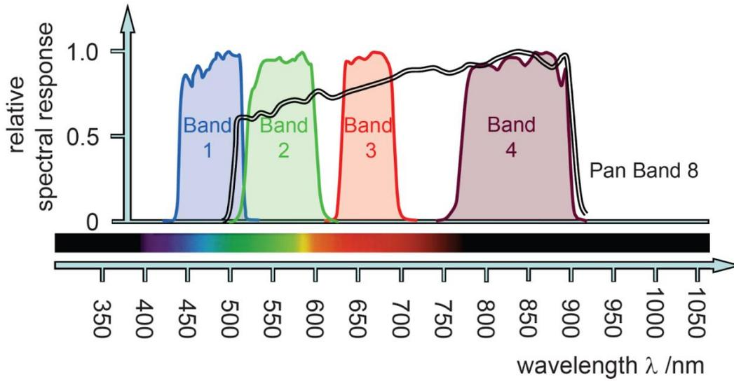
**Figure 8.** Landsat 5 TM and 8 OLI Panchromatic overlapping bands (Source: SEOS)
