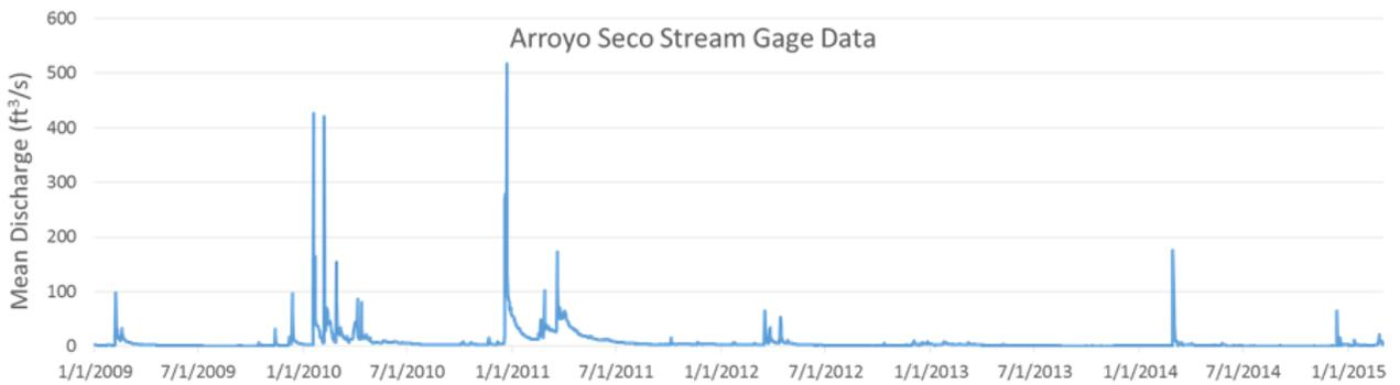
**Figure 2.** Arroyo Seco Stream Gage Mean Discharge vs. Dates
