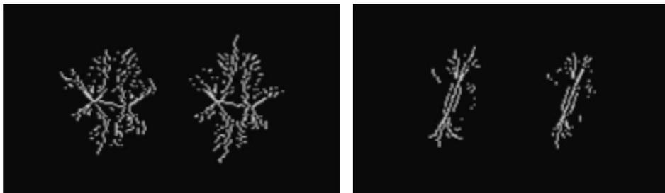
**Figure 18.** Pair of images showing the effects of variations in strike (orientation) on the edge detection algorithm. The faults in this image were modeled in Disloc sharing the same displacement values and geometries but different strikes.
